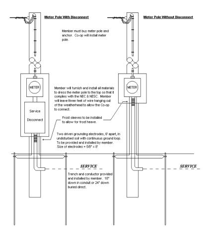
The trench depths specified are minimum and are measured from final grade.
