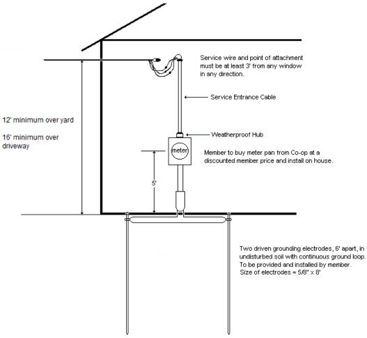
\*Grounding to meet National Electric Code on new construction
