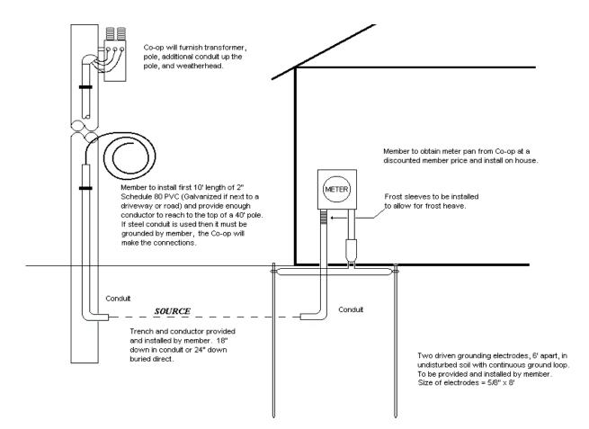
The trench depths specified are minimum and are measured from final grade.
