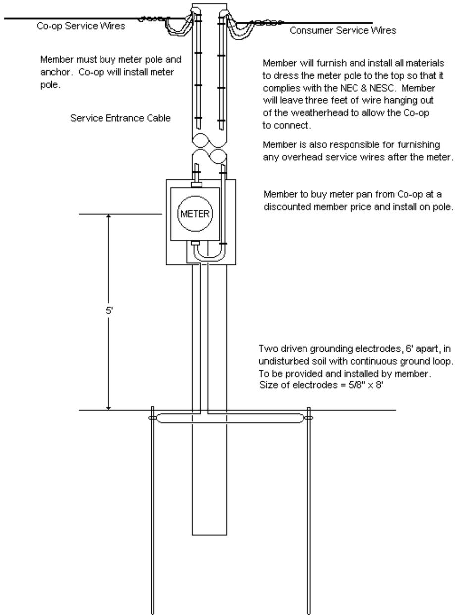
\*Grounding to meet National Electric Code on new construction.
