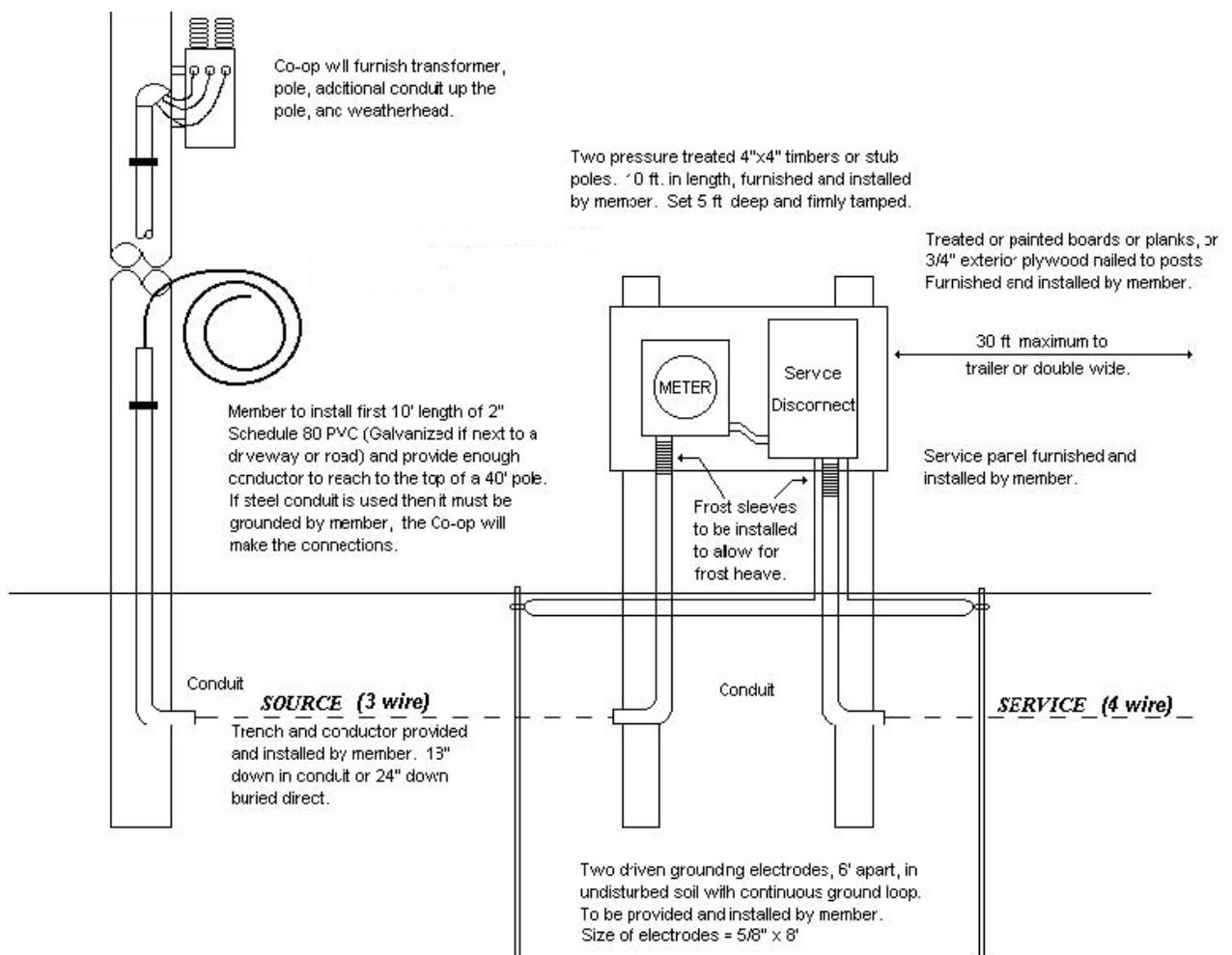
The trench depths specified are minimum and are measured from final grade.
